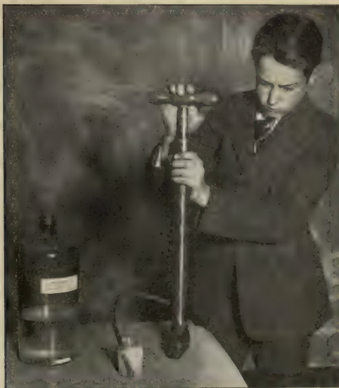
FIG. 189. The limewater test shows that there is carbon dioxid in the air.
